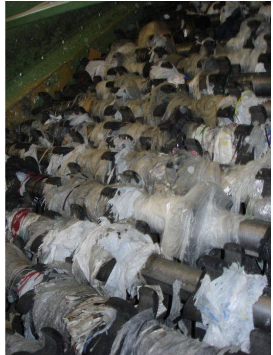
Plastic bags jam the equipment at the Boulder County Recycling Center, just one of the costs the community pays for disposable bag use.
